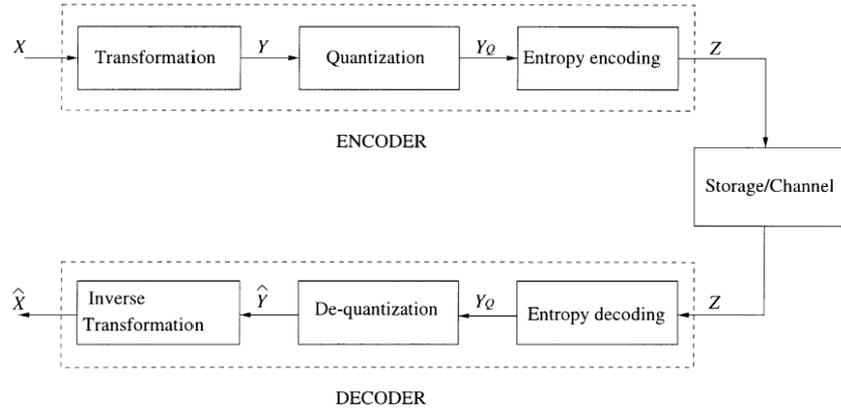
Fig. 1 Block diagram of the general compression and decompression processes [1].
