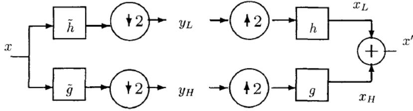
Fig. 3 DWT analysis and synthesis system [5].
