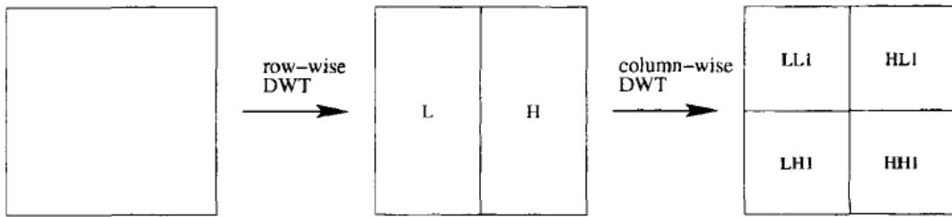
Fig. 5 The two dimensional row and column computation of DWT [5].
