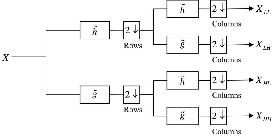
Fig. 4 The 2-D DWT analysis filter bank [1].
