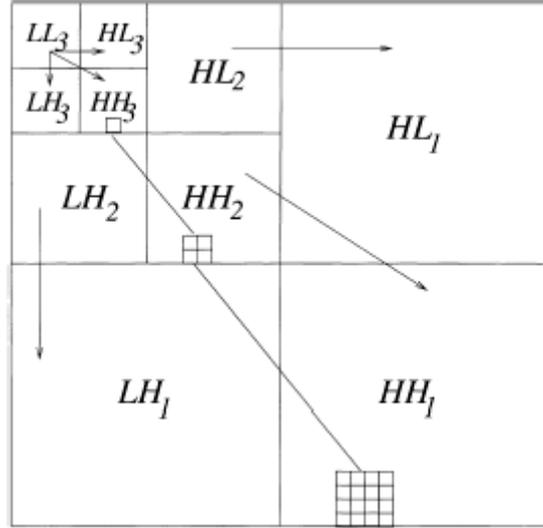
Fig. 7 A three level wavelet decomposition of image spectrum [1].
