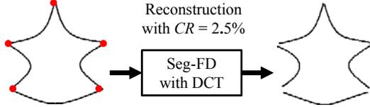
Fig. 9. The illustration of applying the complex coordinates [4] (for shape signatures) and the DCT in *Seg-FD*: The compression rate is 2.5%. Without the end point preserving property, the reconstructed segment is broken at the corners.
