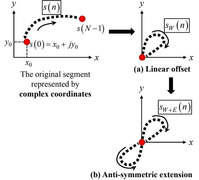
Fig. 4. The illustration of performing (a) *linear-offset* (resulting in a sharp angle at the origin) and (b) *anti-symmetric extension* on a non-closed segment. As shown, the output segment after these two steps become a closed one and has continuous first-order differences at the two end points.
