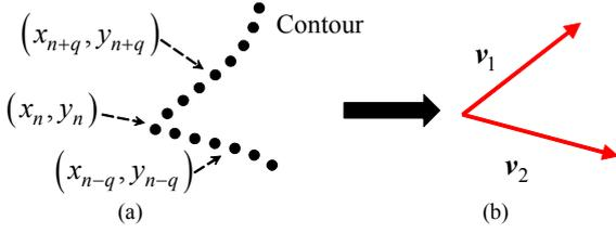
Fig. 8. The corner detection algorithm used in our paper: (a) for each point on the contour, two neighboring points (with  $q = 4$ ) are selected; (b) The two vectors generated by (10) are used to compute the normalized inner product.
