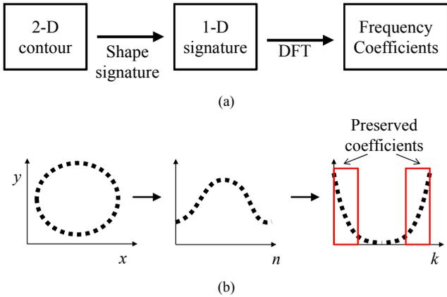
Fig. 2. The general procedure of Fourier descriptors: (a) the flowchart with 2 stages: shape signature and the DFT; (b) an example to illustrate the input and output of the two stages. For efficient recording and description, only the low-frequency coefficients are preserved.
