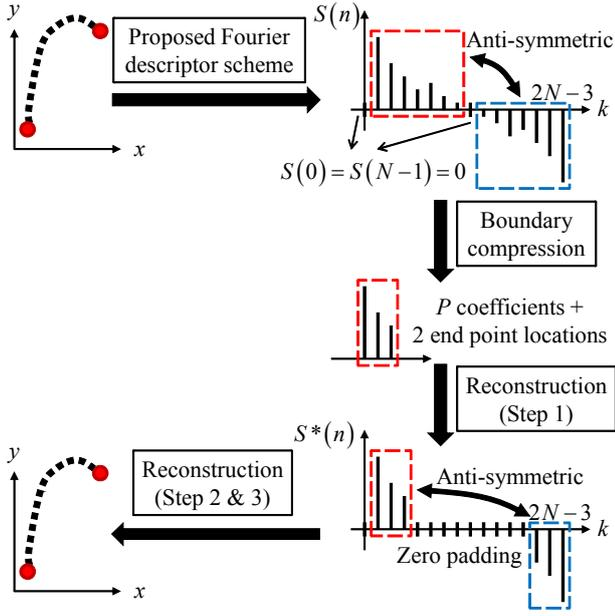
Fig. 6. Illustrations of both the boundary compression and the reconstruction processes: After applying the proposed scheme,  $P$  of the coefficients and the two end point locations are remained for boundary recording. To reconstruct the non-closed segment, we first regenerate the  $(2N-2)$ -long coefficient sequence (Step 1) and then perform Steps 2 & 3 in Section III-D to achieve it.
