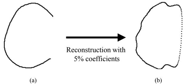
Fig. 1. The problem of using the conventional Fourier descriptor to compress and reconstruct the non-closed segment: (a) the original segment; (b) the reconstruction segment with 5% Fourier coefficients at the low-frequency part. As shown, truncation the high-frequency coefficients results in severe distortion around the two end points.
