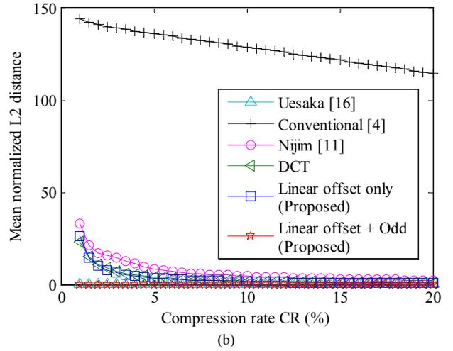
Fig. 11. The average **reconstruction errors** of non-closed segments computed on the MPEG-7 database under varied compression rates: (a) the average normalized  $L_1$  error; (b) the average normalized  $L_2$  error. The proposed methods (linear offset + odd extension) and the DCT methods have the least reconstruction errors.
