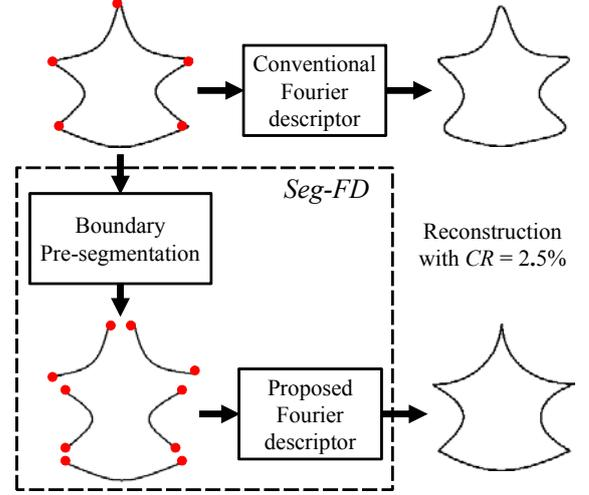
Fig. 7. The flowchart and illustration of the proposed *Seg-FD* framework for closed boundary: The top row shows the reconstruction result using the conventional Fourier descriptor [4] with 2.5% compression rate. The bottom part shows the result of *Seg-FD* (the dash box). As shown, the proposed *Seg-FD* framework could lead to better reconstruction quality, *especially around the corners*.
