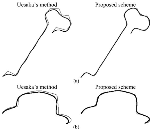
Fig. 17. The reconstruction results of Uesaka's method and the proposed scheme on the non-closed segments used in Fig. 13 at  $CR = 3\%$ . The original segment is plotted in gray color. As presented, Uesaka's method has larger reconstruction error.
