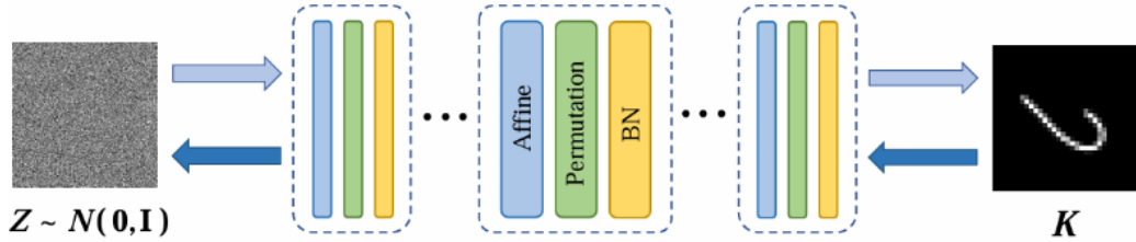
Figure 93: The illustration of the normalizing flow model, each flow block which consists of a batch normalization layer, a permutation layer and a affine transformation layer.
